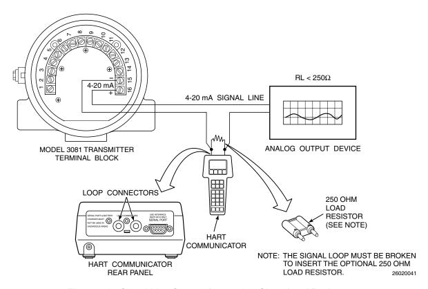
Figure 4-2. Signal Line Connections, < 250 Ohms Lead Resistance
